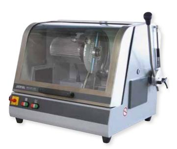
The **BRILLANT 200** is an especially user-friendly wet abrasive cut-off machine with manual cut-off. Opening the machine folds away the hood to the inside so that the whole cutting chamber is easily accessible. The round window opens a wide field of view during the cutting process.
